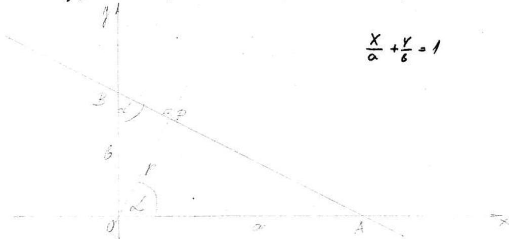
$$\begin{aligned} OPA_{\Delta} \dots \dots \cos L &= \frac{p}{a} \rightarrow a = \frac{p}{\cos L} \\ OPB_{\Delta} \dots \dots \sin L &= \frac{p}{b} \rightarrow b = \frac{p}{\sin L} \end{aligned}$$
